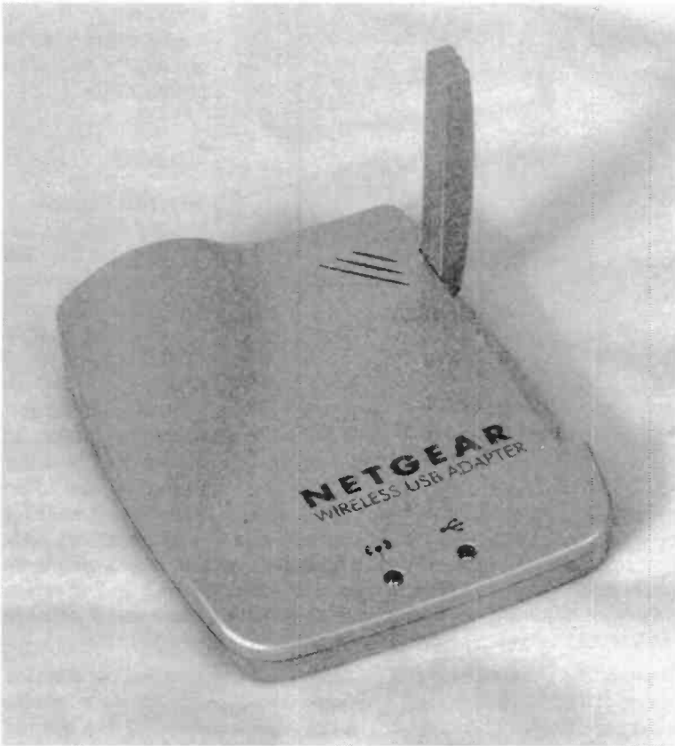
Fig.3.3 This Netgear adapter connects to the PC using an ordinary (A to B) USB cable
