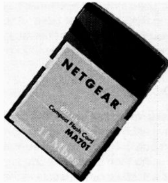
Fig.3.12 This Netgear CF card is actually a wi-fi adapter
