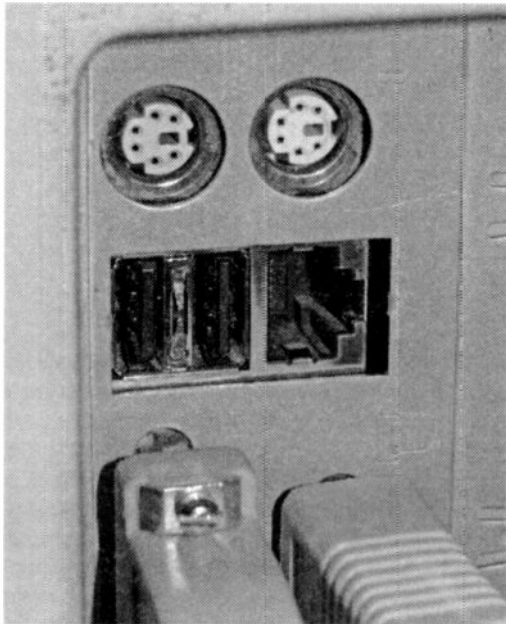
Fig.1.1 The Ethernet port is to the right of the two USB ports
