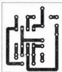
Fig. 2.12 Modulation oscillator PCB toil
