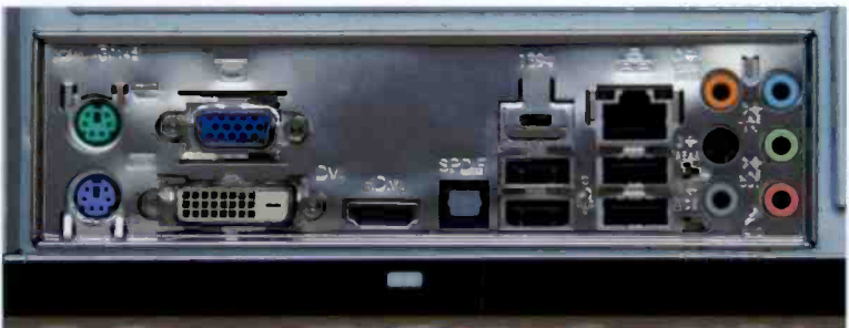
Fig.2.8 Here the plate supplied with the motherboard is in place on the completed PC
