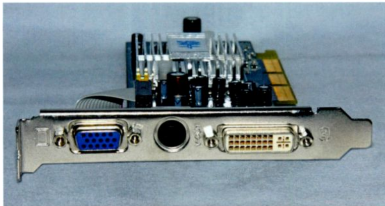
Fig.1.9 This video card has an ordinary VGA output (left) and a DVI type (right)
