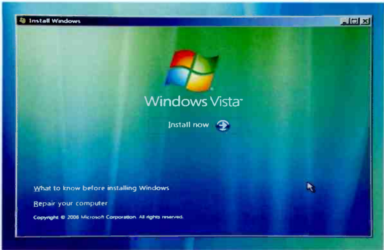
Fig.3.14 It is normally the Install Now option that is selected here. Use the Repair option if you need to make an existing Windows installation usable with the new PC
