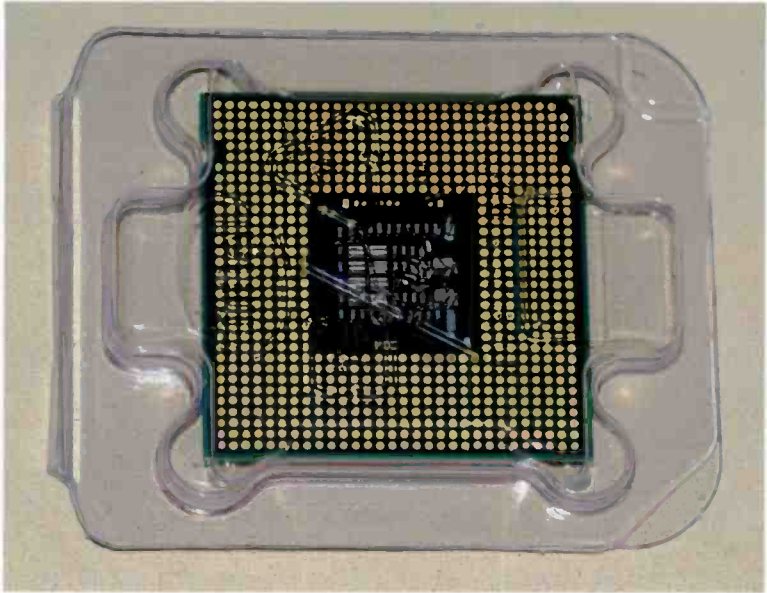
Fig.2.14 The connections on the underside of the processor
