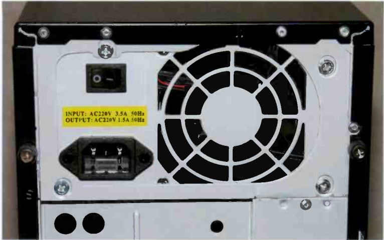
Fig.2.10 The power supply is fixed to the rear panel by four screws
