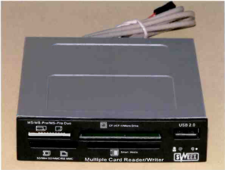
Fig.2.64 This Flash card reader also provides one USB port
