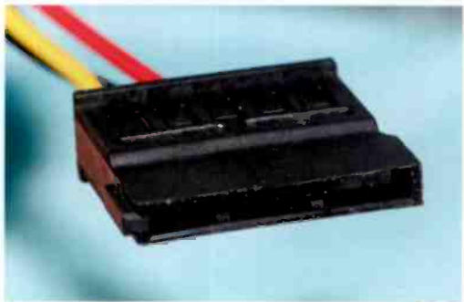
Fig.2.52 The connector on a SATA power lead
