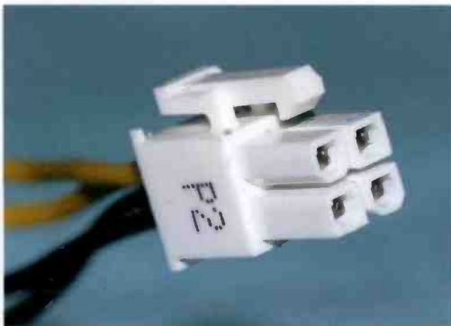
Fig.2.46 There is often an additional 4-way power lead
