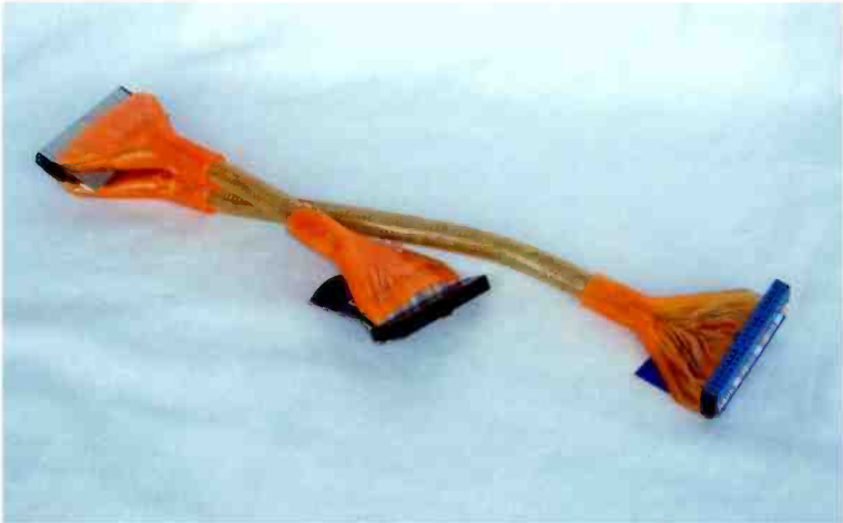
Fig.2.35 The "round" version of an IDE data cable has its advantages
