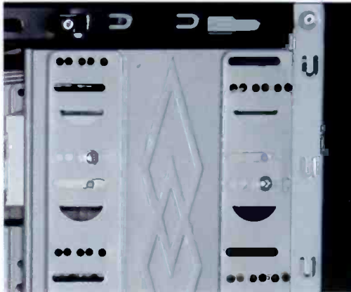
Fig.2.31 Two bolts on each side of a drive are sufficient to fix it reliably
