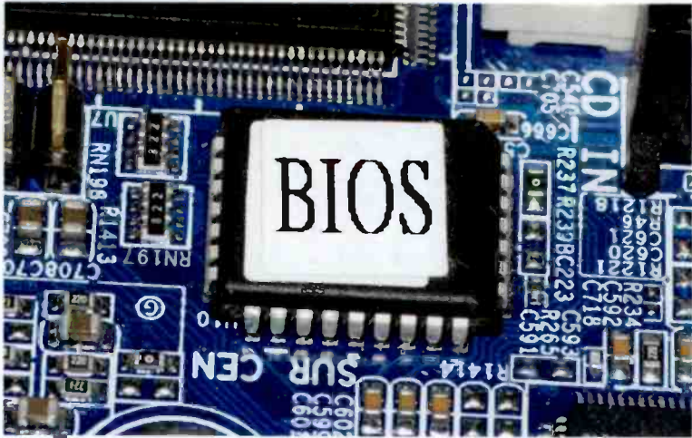
Fig.3.1 The BIOS Setup program is contained in a chip on the motherboard
