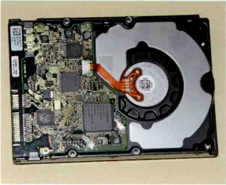
Fig.2.33 The underside of a hard disc drive is usually open, revealing a circuit board and part of the mechanism
