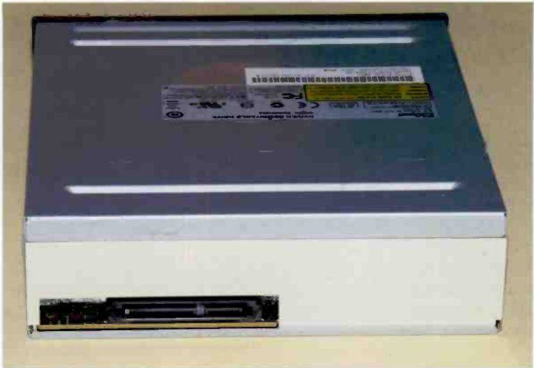
Fig.1.5 The large connector on this DVD drive actually consists of separate power and data ports
