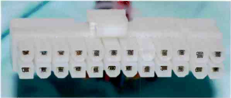
Fig.2.43 A 24-way power connector. The block of four terminals at the right end can be removed to leave a 20-way type
