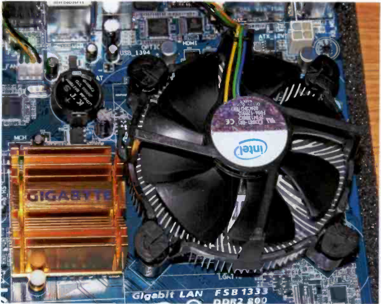
Fig.2.21 The heatsink and fan installed on the motherboard
