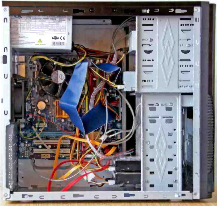
Fig.2.69 The interior of the completed PC. Some tidying of the cables is required
