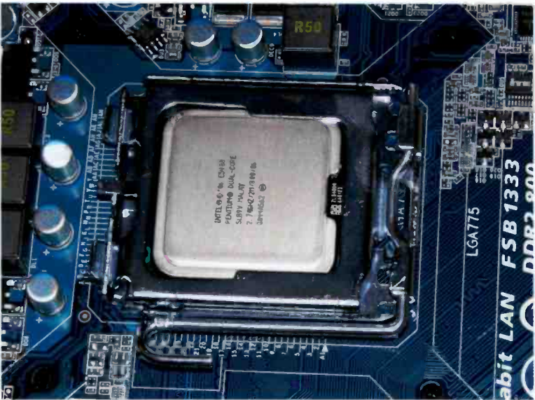
Fig.2.18 The processor has been locked in place
