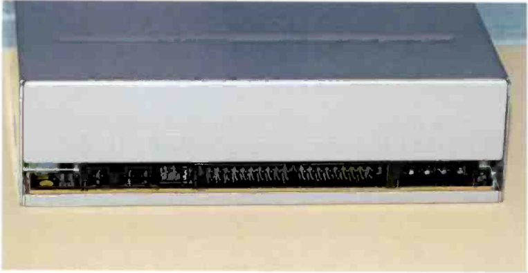
Fig.2.39 The rear of a parallel IDE DVD drive
