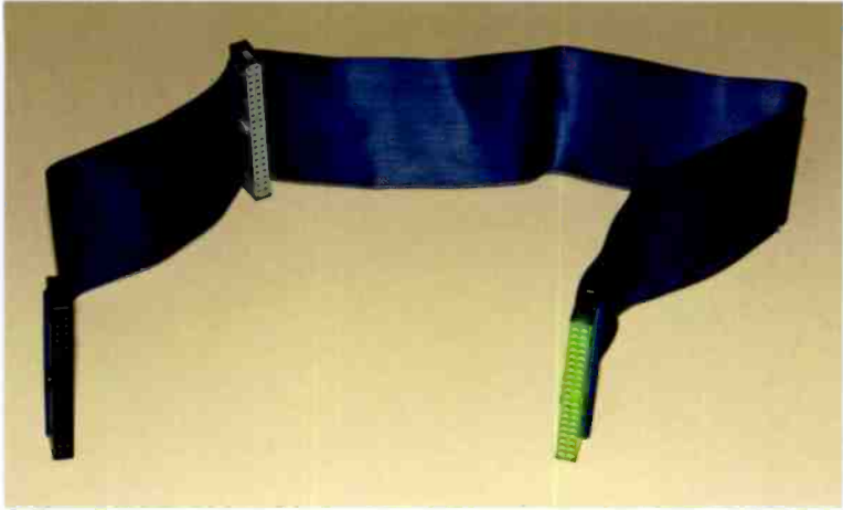
Fig.2.34 A standard parallel IDE cable for one or two drives
