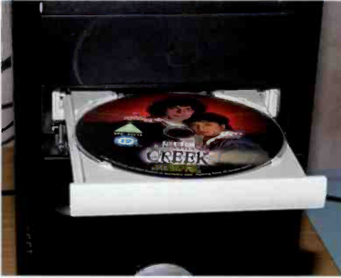
Fig.2.30 The tray has pushed the flap down and out of the way
