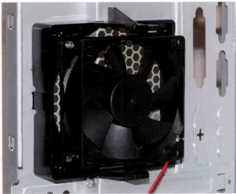
Fig.2.66 A cooling fan mounted on the rear panel of the case. Fans fitted on the side or front panels can be more noisy
