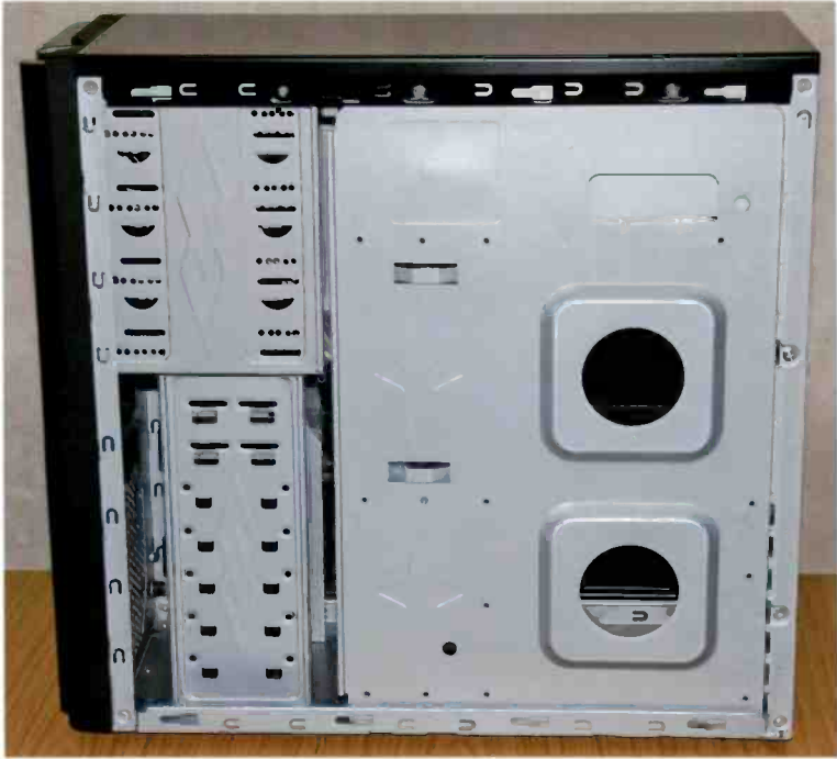
Fig.2.3 The right side of the case provides access to one side of the drive cages, but little else
