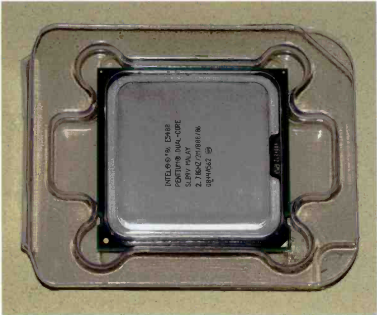
Fig.2.15 The top side of the processor, which is still in its anti-static packing
