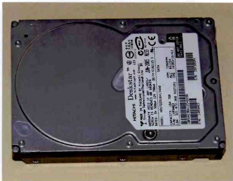
Fig.2.32 The upper side of a hard disc drive is usually enclosed
