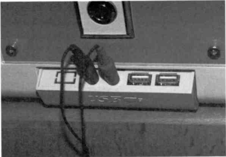
Fig.1.30 There will often be headphone and microphone sockets on the front panel
