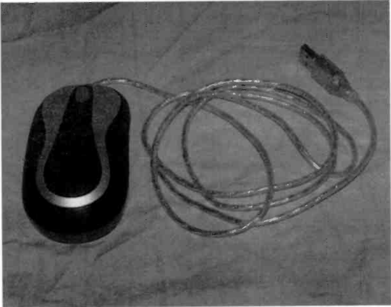
Fig.1.5 These days many mice connect to a USB port rather than the PS/2 mouse port
