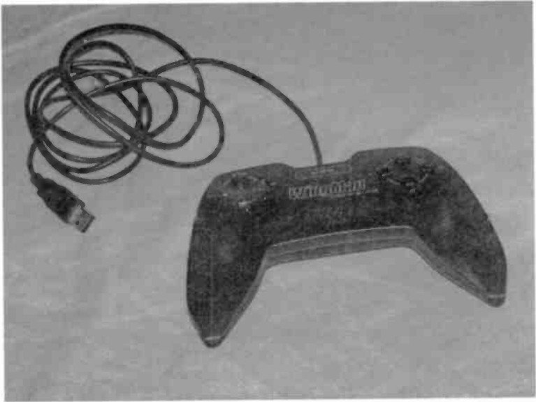
Fig.1.27 These days most games controllers, like this one, connect to a USB port
