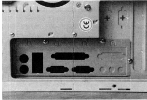
Fig.3.7 The new port cover plate installed on an ATX case
