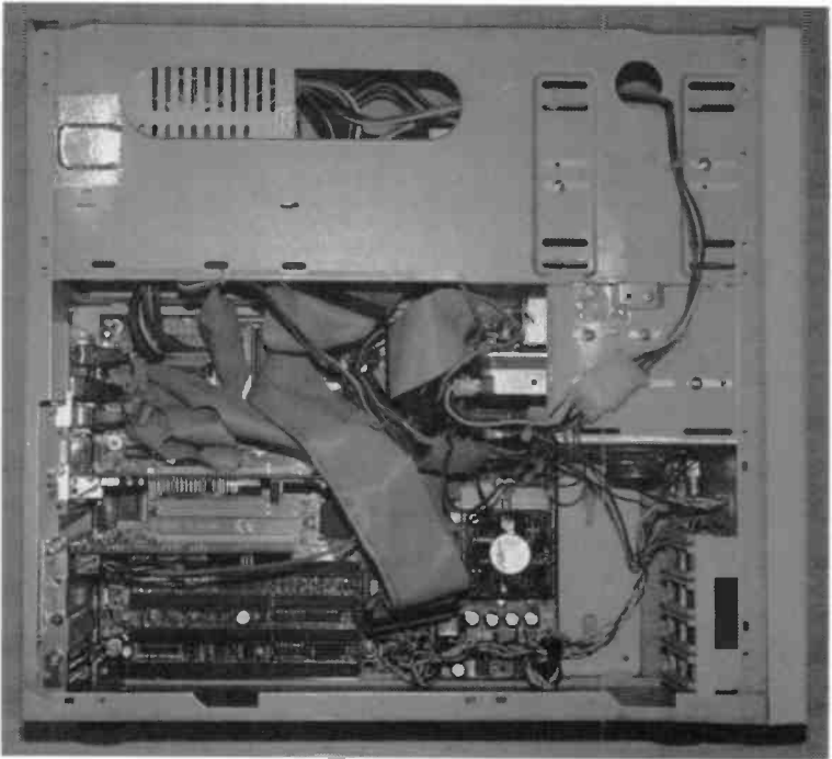
Fig.3.39 It is a good idea to tie down some of the cables in the finished PC
