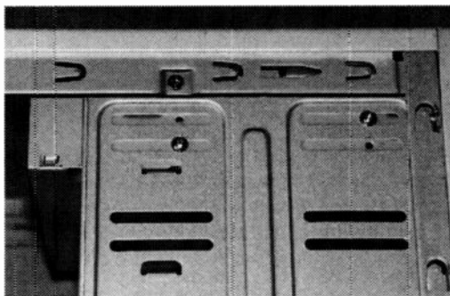
Fig.3.28 Two fixing screws per side will hold a drive in place
