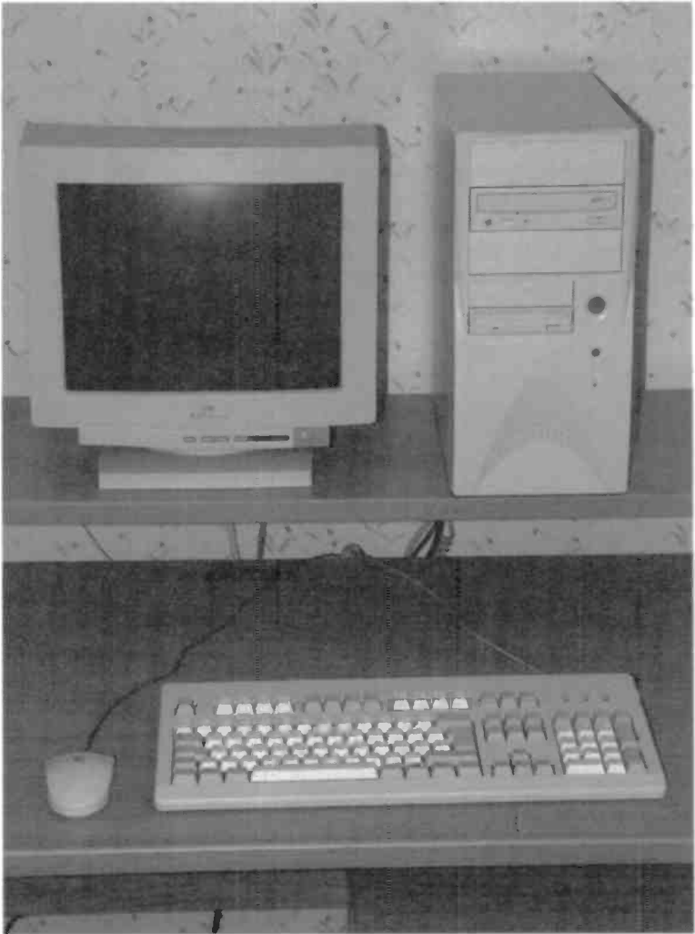
Fig.6.16 A completed and working budget Socket 7 PC. The CD-ROM drive on this one was reluctant to operate due to its loose fitting data cable, but a change to a different cable cured the problem
