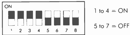
Fig.3.16 An explanatory diagram for DIP-switches
