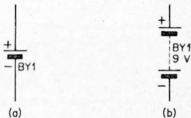
Fig. 13. (a) Circuit symbol for a single cell. (b) Circuit symbol for a multiple cell battery.
