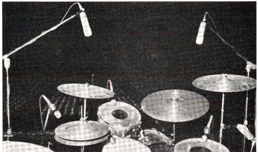
Mike arrangement of John Bonham's kit showing correct positioning.
