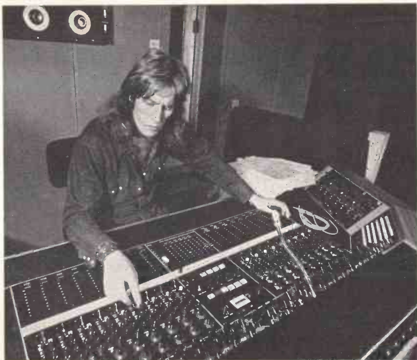
24 Channel, 16 track recording console built for Alvin Lee Ltd.
