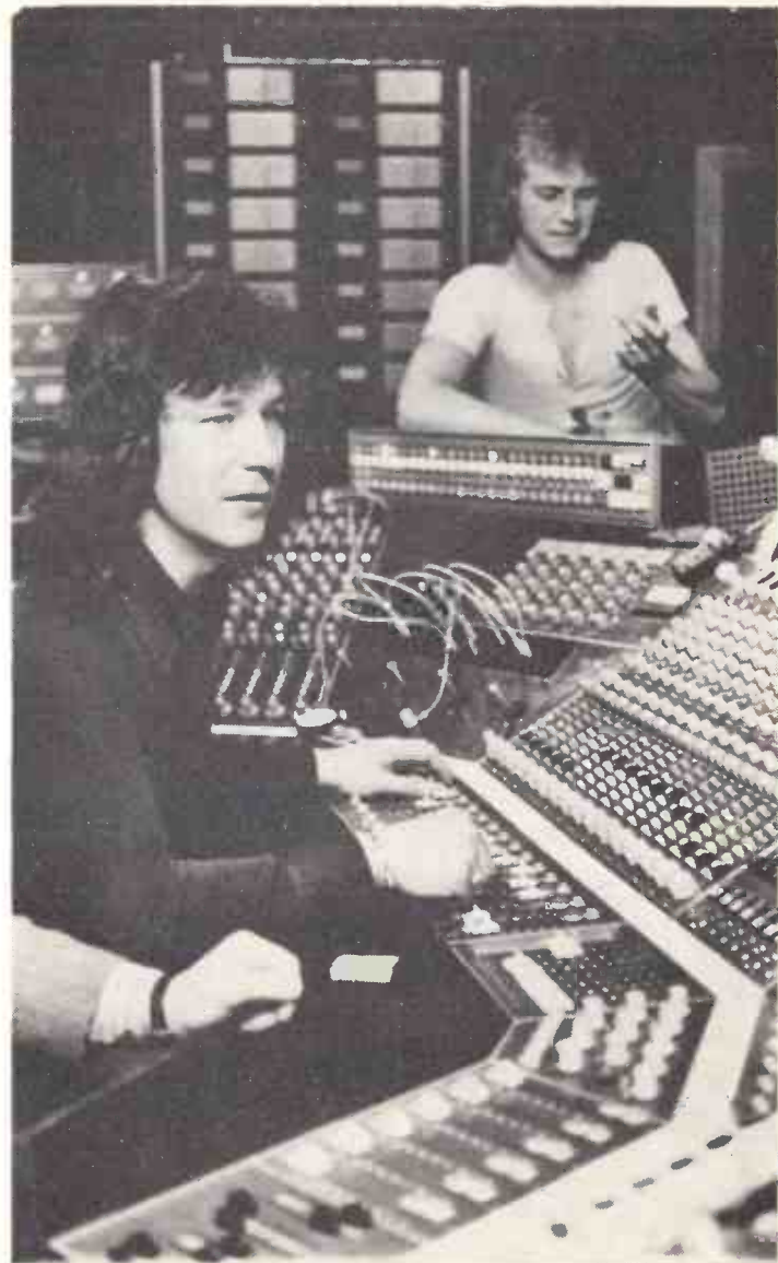
The Helios 32-channel quad desk installed at Ramport Studios
