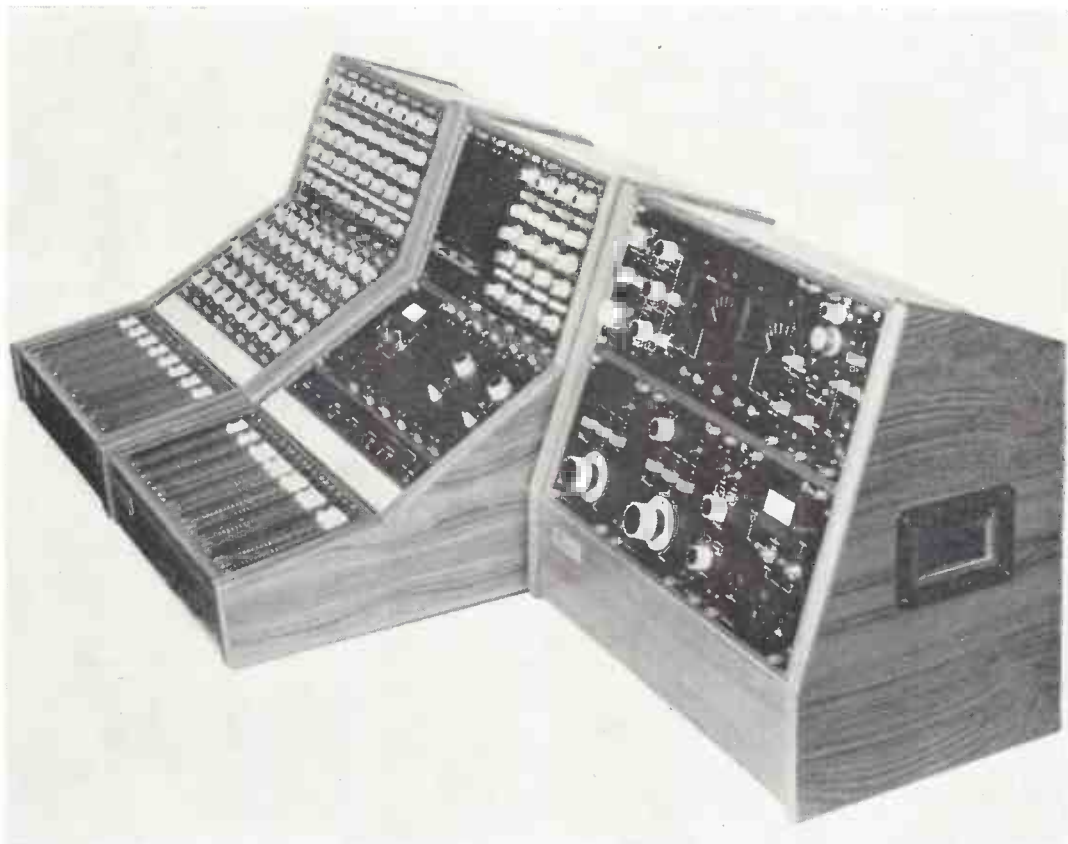
The first delivery of stereophonic outside broadcasting equipment has been delivered to the BBC by Calder Recordings Ltd. It is the first stereo unit the Corporation has had and was demonstrated recently at the Audio Fair in London. The system, pictured above, is in three operational units, consisting of an eight-channel input with full equalisation on each channel, in group unit with four auxiliary groups and two echo groups, plus a metering and output unit.
