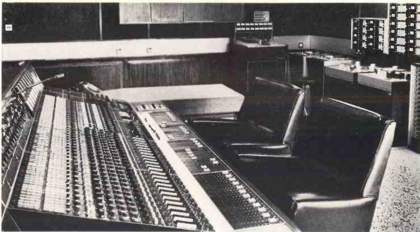
The main control room at AIR with 24 input and 16 output channel Neve desk. Also Dollys and Studers.
