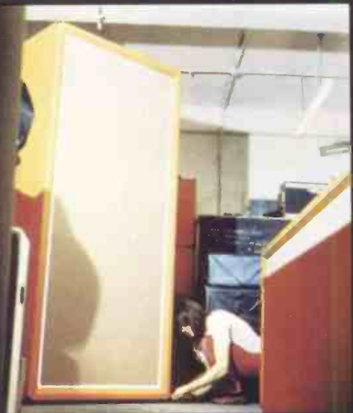
Possibly the largest guitar amplifier cabinet in the world weighing half a ton and incorporating 24 12" speakers.
