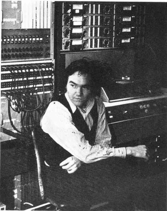
Richard Olsen listens to a playback. Behind him, to the left is the Dolby noise reduction system; on the right is the Ampex 16-track
