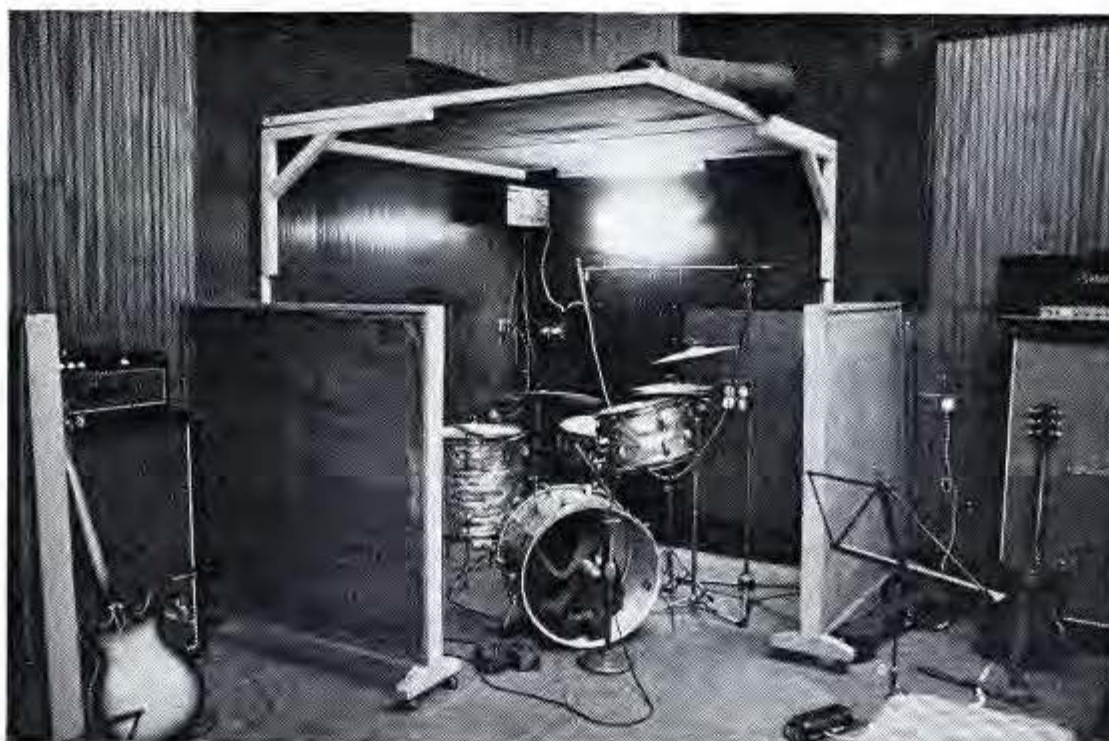
The recording booth for drums at Pye's studios, and those for bass and guitar on either side
