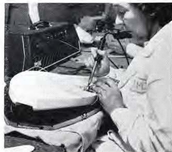
Soldering the electrical circuits in a Phantom body, which is laying on one of the special jigs.
