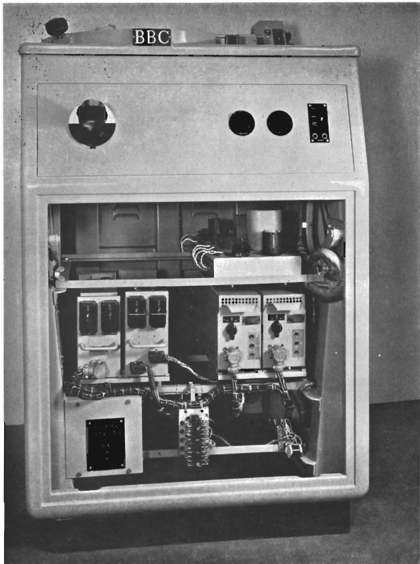
BBC disk reproducing desk Type DRD/1. Control panel (left to right): Main fader, equaliser control, variable attenuator (0-20 db) control monitor key Top deck: Equaliser-attenuator Lower deck (left to right): Mains units, amplifiers
