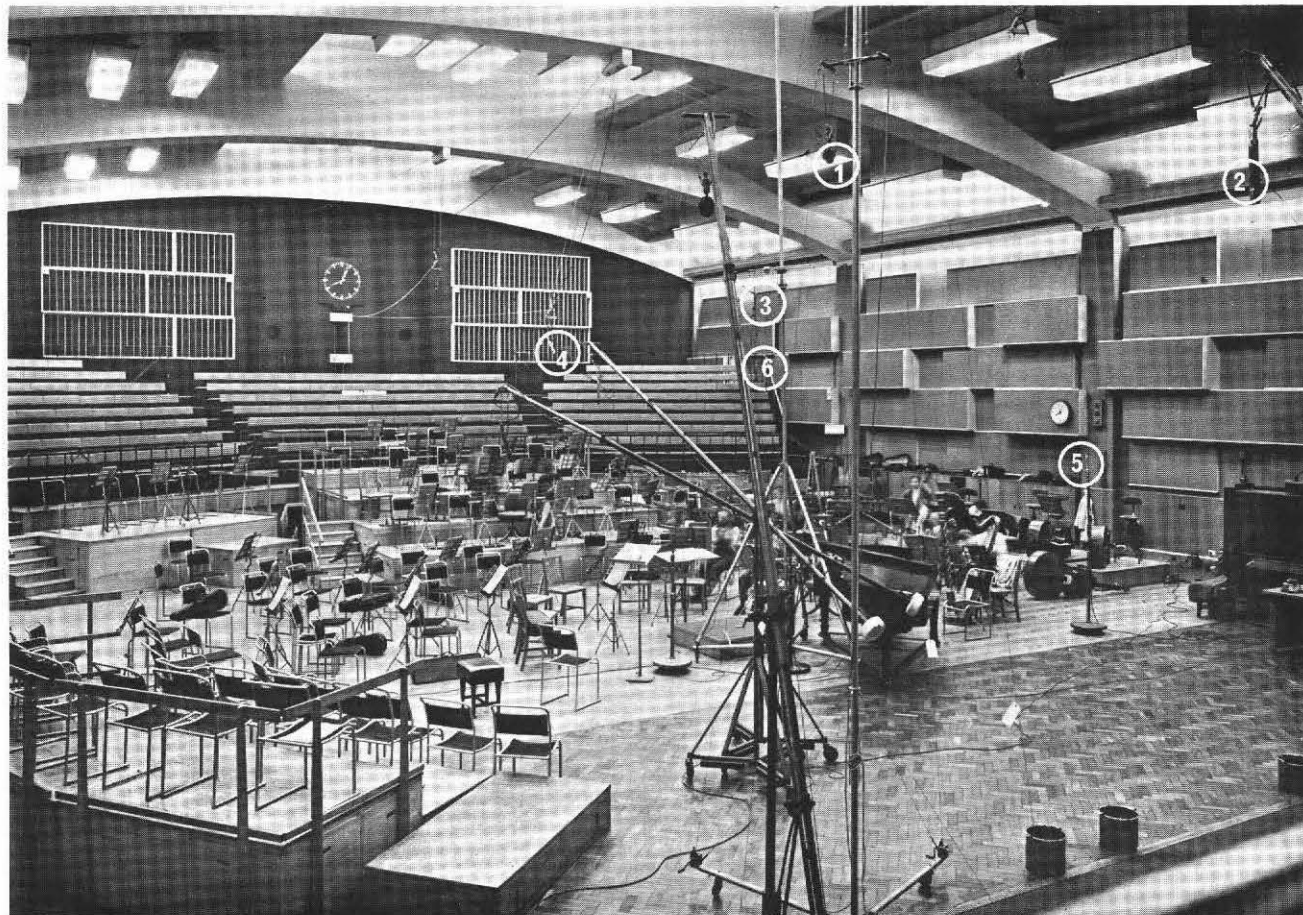
Fig. 3 — Photograph of Maida Vale Studio 1 showing the microphone positions used in the pilot experiment
