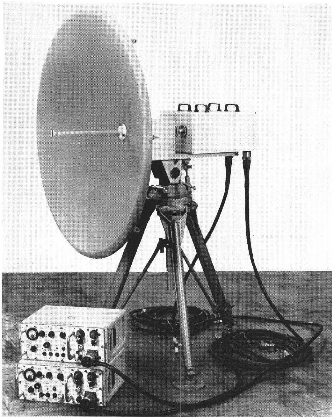
Fig. 4 General view of modern portable link terminal complete with 1.2 m diameter aerial
