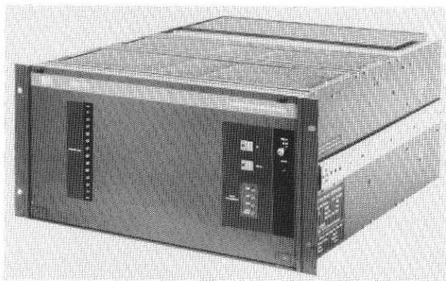
Fig. 1(b) Production version of noise reducer manufactured by Pye TVT. This equipment has recently been brought into service at the network output of BBC-1.
