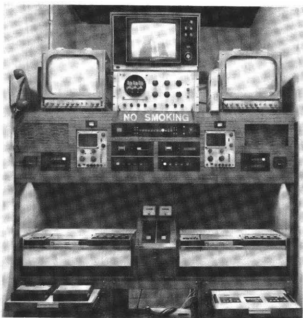
Fig. 3 The videotape area with two cassette machines and full monitoring and editing facilities. The machines can be operated locally or remotely controlled from the studio.
