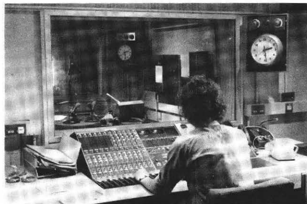
Fig. 6 The control desk in one of the control cubicles. The small talks studio can be seen through the window behind the desk.
