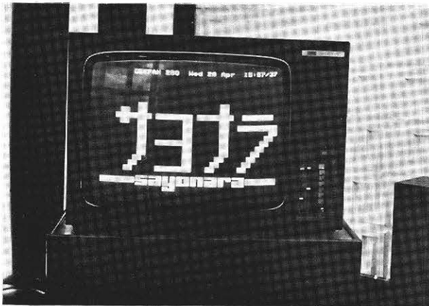
Fig. 3 Although designed to generate the Roman alphabet, CEEFAX can display other shapes by means of its graphics mode of operation
