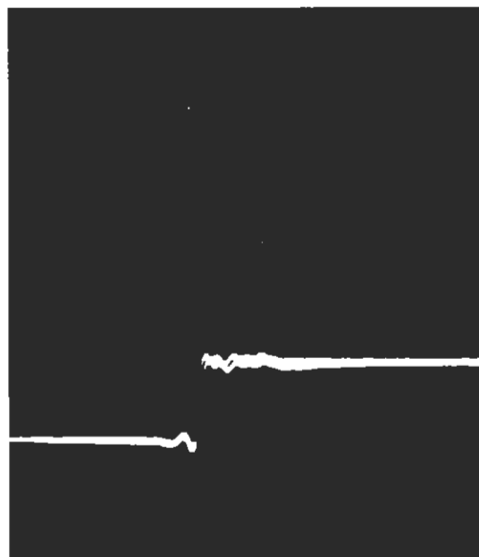
Fig. 9 — Displacement of triggering point of successive lines due to small amount of added hum
