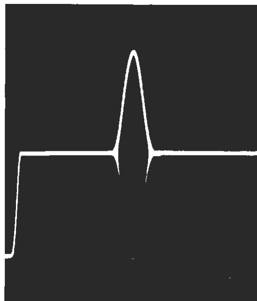
Fig. 2 — Superposition of luminance and chrominance pulses
