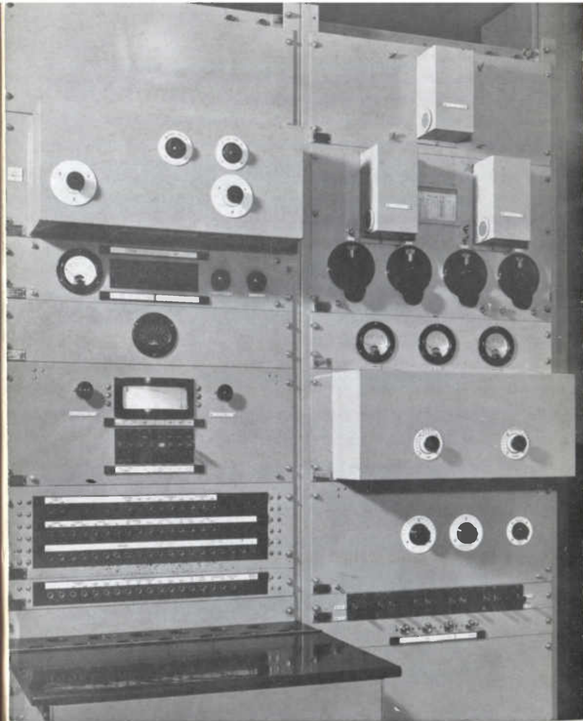
A.C. testing equipment, showing T.P.M., T.M.S., oscillator and amplifier, amplifier detector, and variable attenuator
