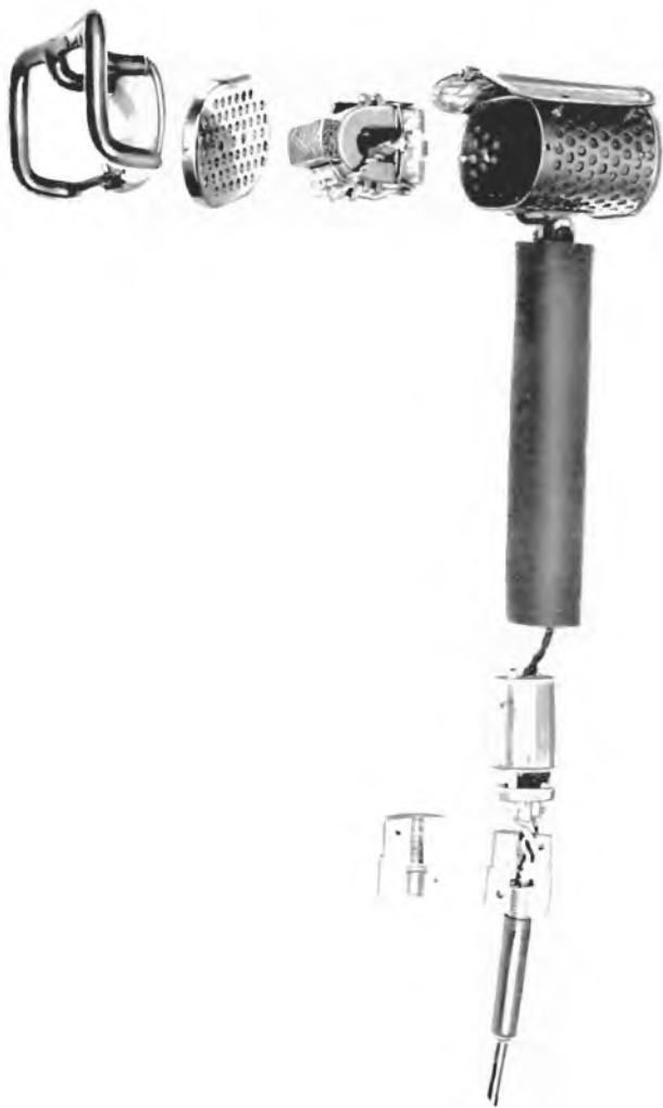
Plate 10.2.—Exploded view of commentator's microphone showing lip-guard microphone inset and breath shields
