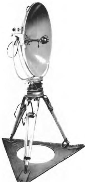
Plate 11.2.—Paraboloid reflector microphone used for outside broadcasts
