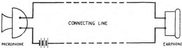
FIG. 32. A SIMPLE, ONE-WAY, TELEPHONE CIRCUIT
