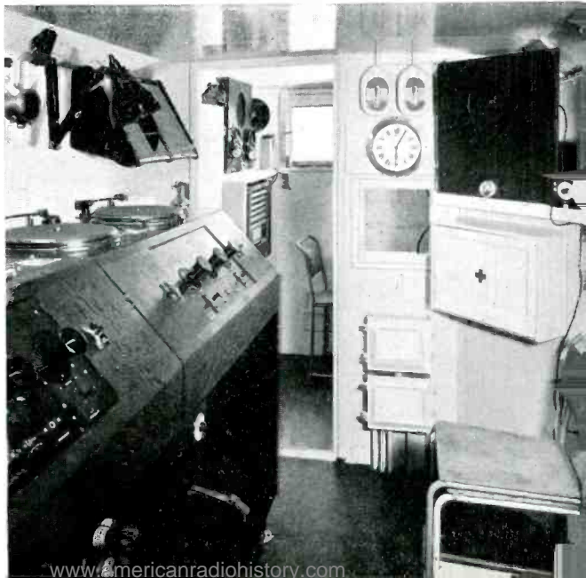
In the mobile studio and reproduction unit ; this shows the reproducing desks and part of the control room
