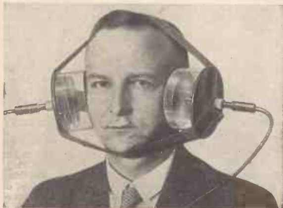
This curious headphone arrangement is used now for treatment of the maxillar-cavity by ultra-short-wave therapy
