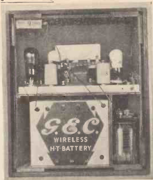
Completely self-contained, the Goodwill Three is a detector and low-frequency amplifier set working from batteries. The design is a simple metal baseplate
