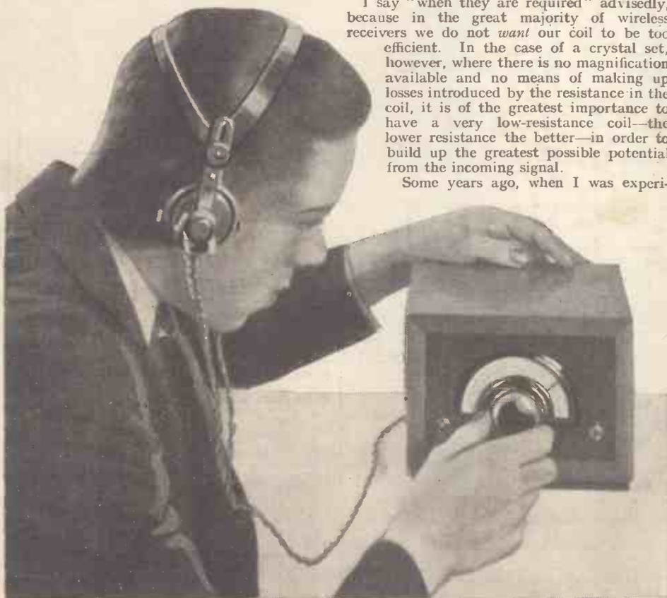
This is one of the most popular crystal sets we have introduced in "Amateur Wireless"—the 150-mile model, designed by Kenneth Jowers and fully described in the October 27 issue. A fine set for Droitwich reception at distances up to nearly 250 miles
