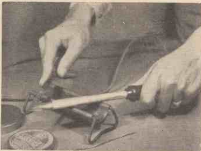
Another picture, taken in our own workshop, showing the all-important job of cleaning the soldering bit—ready for the next and equally important step of tinning the bit
