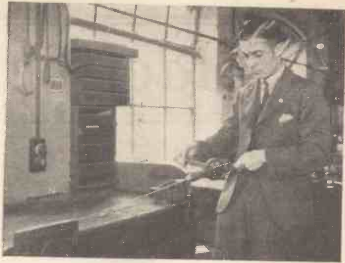
All you need to make these wire-wound condensers are vice, twist drill and suitable wire—plus a little patience!
