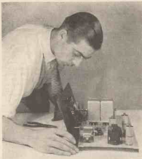
Fitting the ebonite panel to the metal baseplate in an experimental model of the All-Britain Three. Note the use of single tuning condensers, which persist in the final model to be described next week
