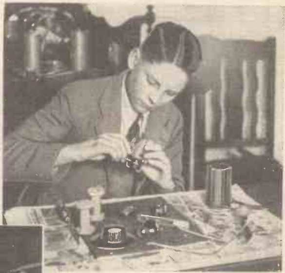
1.—Starting construction of the one-valver to pick up America. Both the coil and the high-frequency choke can be made at home
