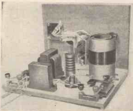
Note how straightforward is the assembly of the Lucerne Minor—a two-valver that can be built for 27s.
