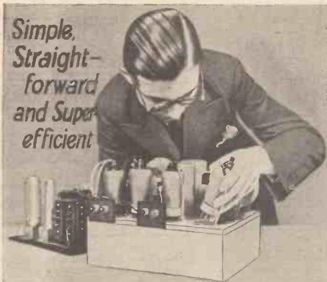
Putting the valves in the 1934 A.C. Century Super, which closely follows the original battery version. Note the mains unit on the left
