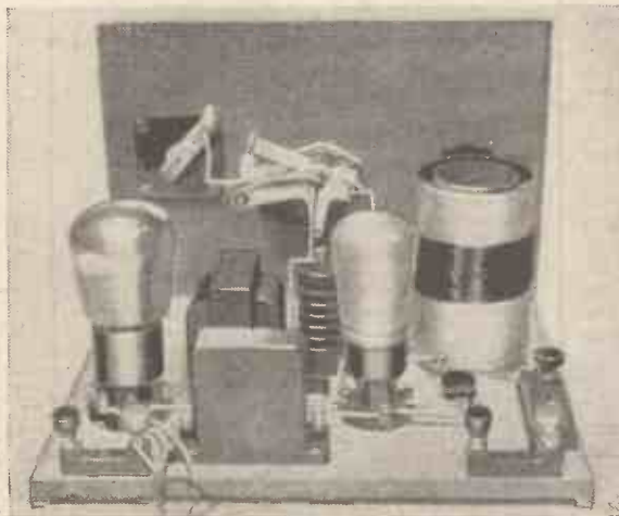
Here is the set with the valves in position all ready for use. A full-size blueprint appears on the inside covers
