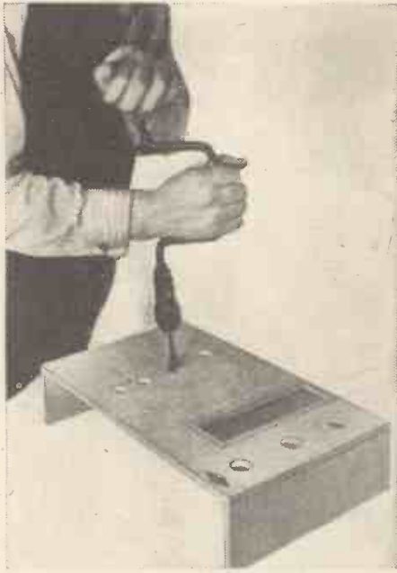
Using a brace and bit to cut a chassis hole
