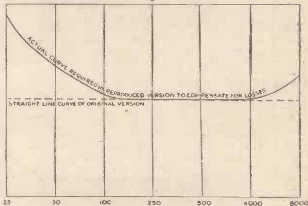
Fig. 3.—This is the kind of frequency-response curve that a good-quality domestic receiver should give
