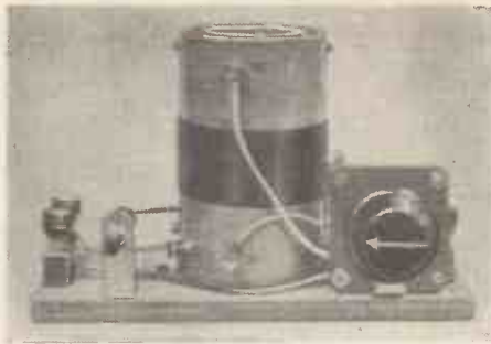
(Above) Another view of the Four-station Crystal Set, which can be made at home very easily; the coil can be home-wound or bought complete if desired. (Right) Theoretical circuit of the set; compare this with the wiring guide
