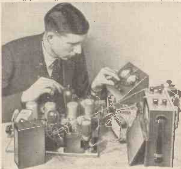
Measuring the anode-current consumption of a set in the AMATEUR WIRELESS laboratories
