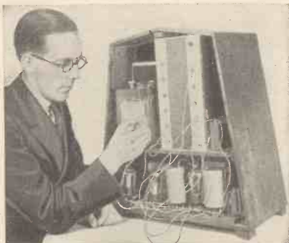
Many people economise in high-tension consumption by plugging down on their anode battery
