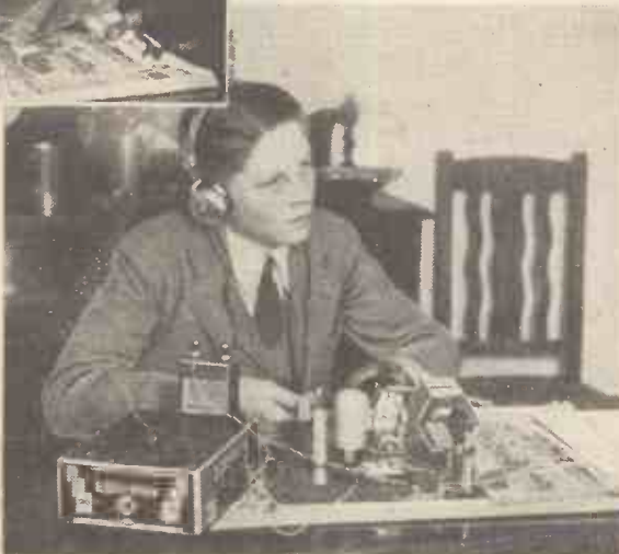
4.—Ah, here we are! The set finally completed and all ready for long-distance reception. It must be used with phones, of course, and will not drive a loud-speaker
