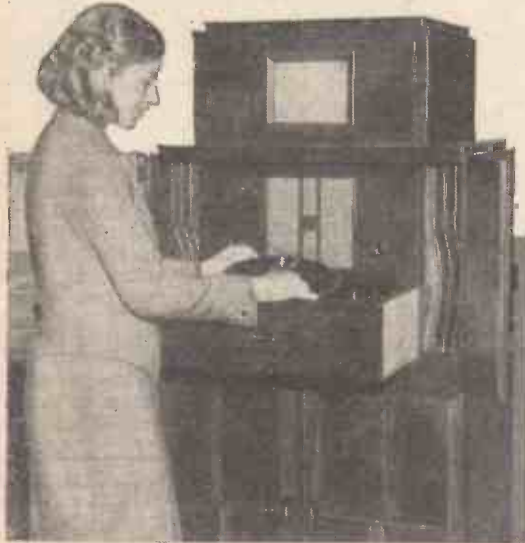
The Telefunken combined television receiver and radio-gramophone shown in Berlin. The cathode-ray tube at the top handles the latest 180-line 25-frame transmissions
