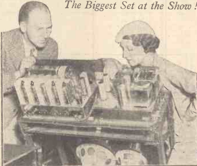
Two visitors at the Radio Show examining the new R.G.D. twelve-valve super-het chassis. Note the Catkin valves in the set and the dual loud-speakers at the bottom of the picture
