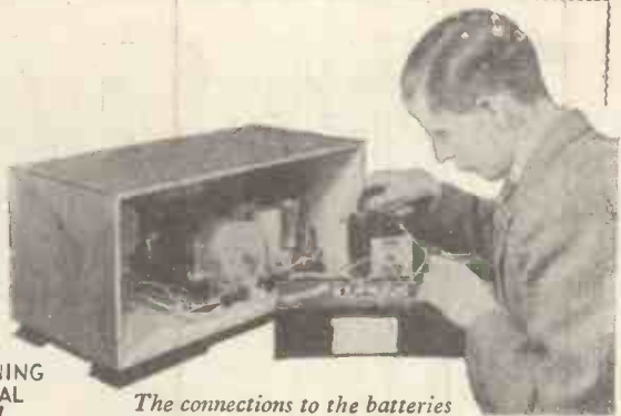
The connections to the batteries can be easily seen from the blueprint. H.T.+1 should be plugged into the 60-volt and H.T.+2 into the maximum tapping of the high-tension battery
