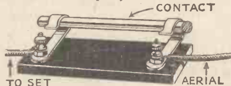
An old grid-leak holder brought into service as a simple aerial-earthing switch
