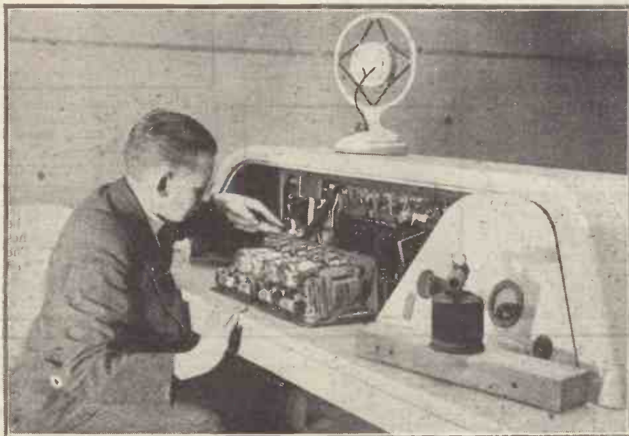
Probing into the mysteries of the D. C. P. Every piece of B.B.C. apparatus has to be regularly tested and here an engineer is seen examining the wiring of a dramatic control panel
