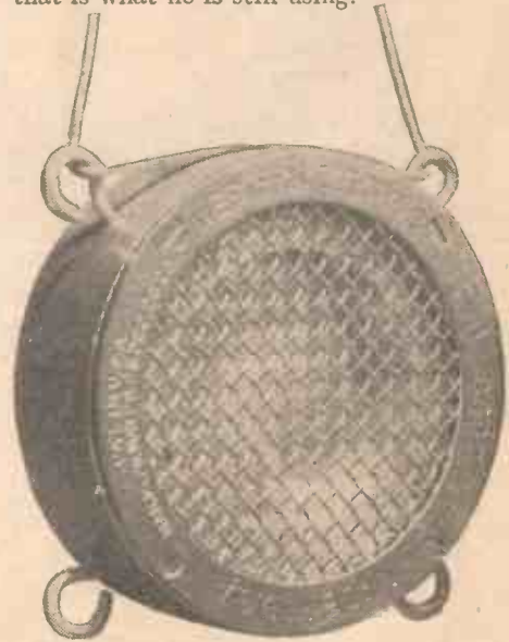
One of the Western Electric microphones. This type is generally used with a baffle
