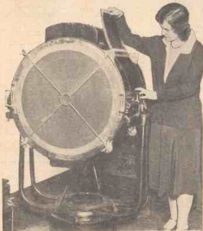
What is claimed to be the largest cone speaker in the world is this new directional "searchlight" speaker which can be heard three miles away
