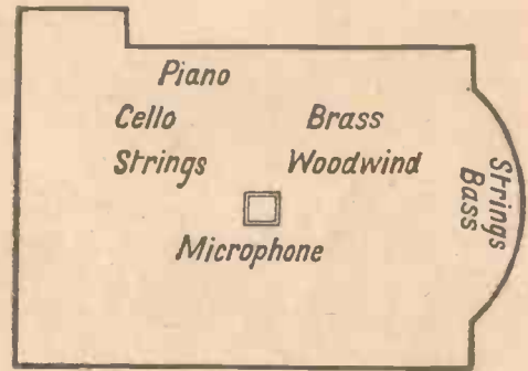
This plan gives a good idea of the instrument arrangement at a typical cinema orchestra broadcast—from the Commodore Theatre, Hammersmith
