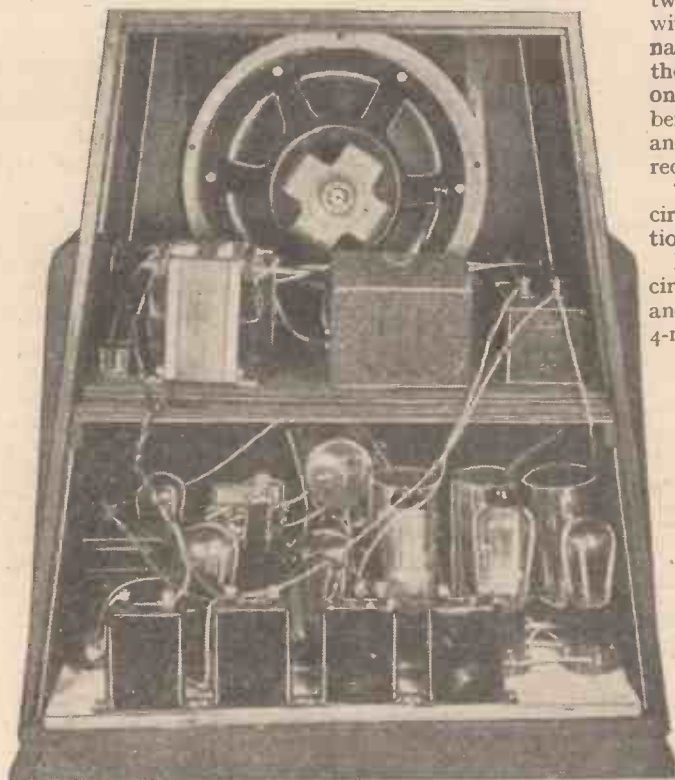
This picture of the interior shows how the receiver and mains unit are housed in the cabinet
