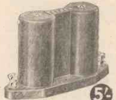
The Telsen Binocular H.F. Choke has an exceptionally high impedance and low capacity resulting in an excellent performance curve. It has a restricted field and covers the whole broadcast. Free from parasitic resonances. Inductance: 180,000 microhenries. Self Capacity: .000002 microfarad, Resistance: 750 ohms. Price 5/- each.
