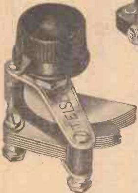
TELSEN VARIABLE CONDENSELS (bakelite dielectric). Particularly designed for use as a reaction condenser. May also be used as a neutralising condenser where large capacity is necessary. All vanes are insulated with bakelite. Made in three capacities: .0005, .0003, and .00015. Supplied complete with pointer knob, with one-hole fixing for panel mounting. Price 3/- each.
