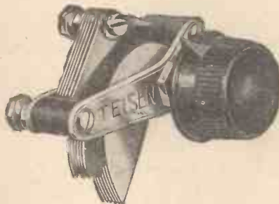
Telsen Variable Condensers (bakelite dielectric). Particularly designed for use as a reaction condenser. May also be used as a neutralising condenser where large capacity is necessary. All vanes are insulated with bakelite, which eliminates the possibility of a short circuit between the moving and fixed vanes. Made in three capacities: .0005, .0003, and .00015. Supplied complete with pointer knob, with one-hole fixing for panel mounting. Price 3/- each.
