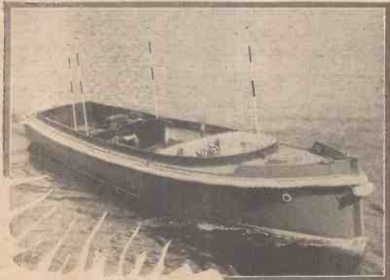
A "close-up" of a radio-controlled motor launch which appeared in Portsmouth Dockyard during Navy Week. The aerial is supported by the posts at the stern.
