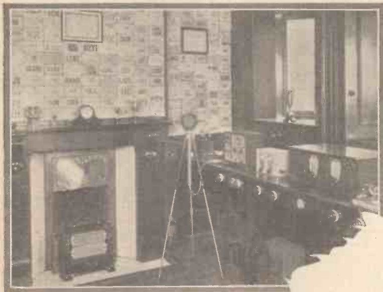
A peep into a well-known amateur station G5BY. The Philips microphone in the foreground is of the type used at Hilversum and Hulzen. On the bench are the receiver and speech amplifiers
