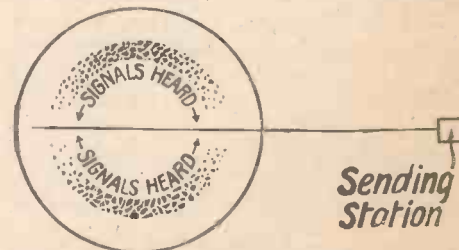
Diagram showing how the strength of the received signal varies according to the position of the frame aerial
