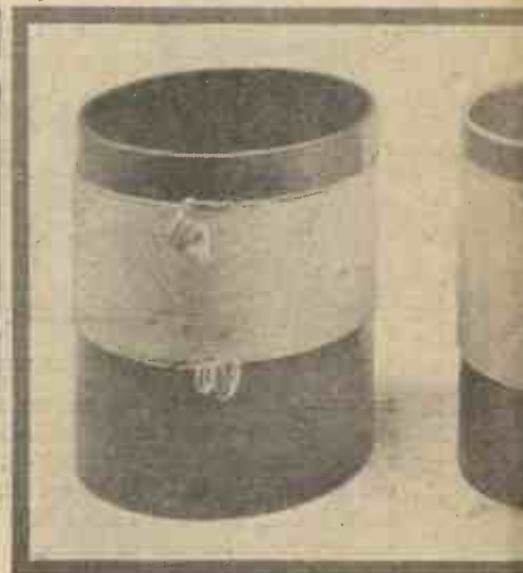
Coils Nos. 1, 2 and 3, 3 in., 2 1/2 in. and 2 in. value—viz., 200, 100, and 50 microhenries
