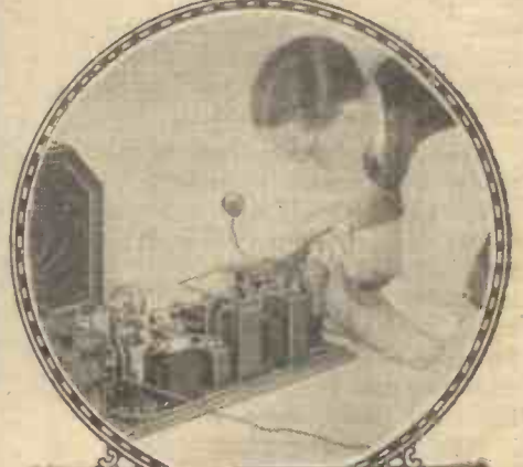
A dangerous practice is to work with metal tools in the set while the batteries are connected up, or if the receiver is of the mains-operated type, while the current is switched on.
