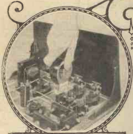
The only serious wear to which a plug-in coil is usually subjected is that due to careless plugging in or pulling out. If you wish your coils to last you should always handle them by the base.
