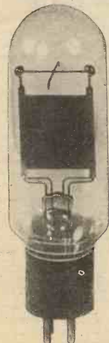
The Raytheon neon tube as used for television purposes
