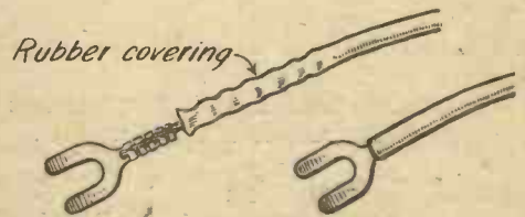
Method of Making Neat Flex Leads.
