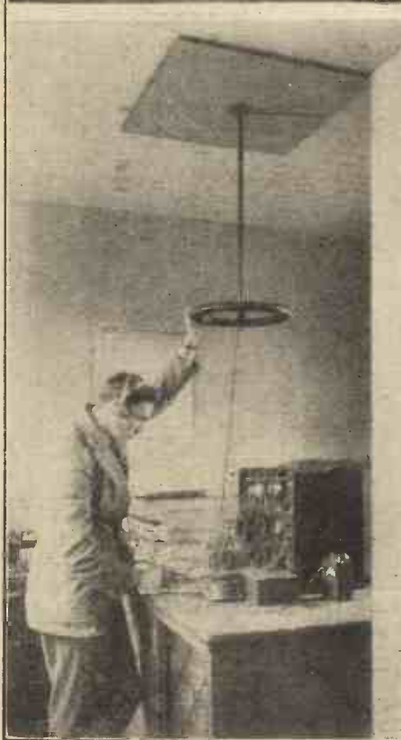
A Complete Experimental Direction-finding Apparatus in use at Croydon Aerodrome.
