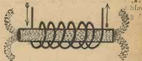
Fig. 3.—Increased Effect by Use of Iron Core.
