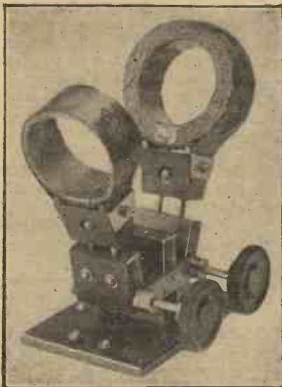
Fig. 7.—Honeycomb Coils in Use as Tuner.
