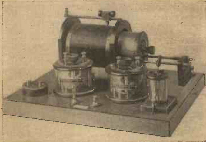
A Crystal Receiving Set with Loose Coupler.
