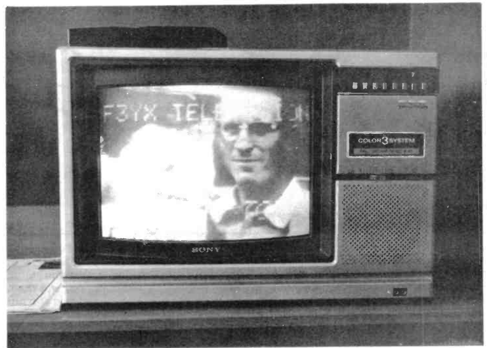
Crossband 24/70cm working adds a new dimension to ATV. Here F3YX is relaying on 438.5MHz a signal received on 1255MHz from F1MV. These transmissions were picked up by F1DL who in turn relayed them on 1255 to F1BJB who made this recording
