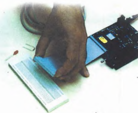
Fig. 6 - Colocando o DIP 40 no Proto Board.
