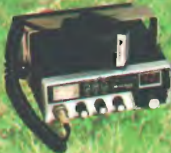
rtx mobile 5W AM 40 canali mod. 150 M
