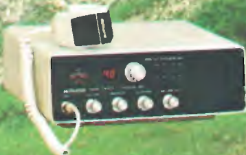
rtx base 5W AM 15 W SSB 120 canali (40ch. AM - 40ch. LSB - 40ch. USB) mod. 76534
