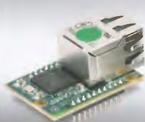
Nano LANReach™ Nano SocketLAN™ 805,- / 785,- Kč UART, SPI, USB, RMII LAN: RJ45
