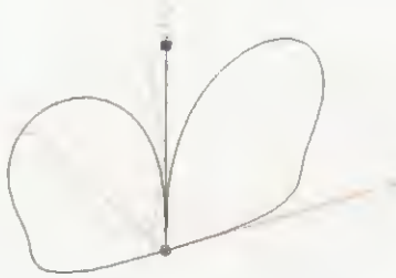
Obr. 4 a. MW, h = 5 \text{ m} , whip = 0,1 m, f = 30 \text{ MHz}
