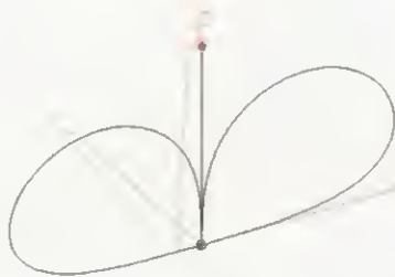
Obr. 3. MW, h = 5 \text{ m} , whip = 0,1 m, f = 10 \text{ MHz}
