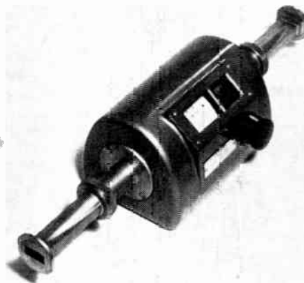
Figure 4. An X-band rotary attenuator by Elliot Brothers (London) Ltd. Unit may be used with either rectangular or circular waveguides . . . employs a rotating glass absorptive vane . . . can be used as a rotary phase-shifter.
