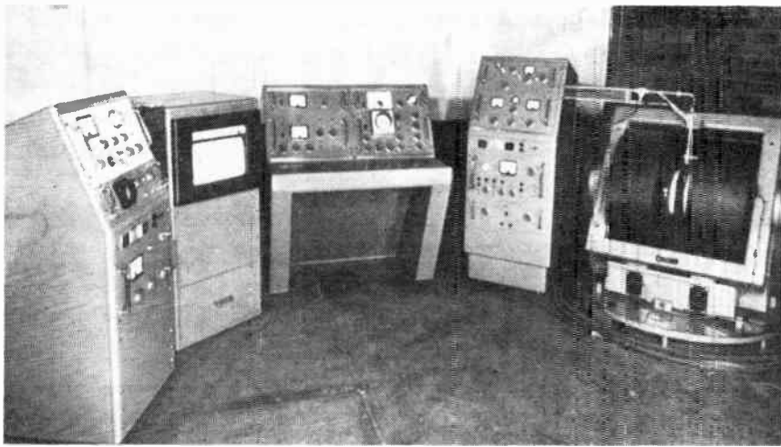
Figure 2. The Hilger and Watts 8 mm electron spin resonance spectrometer.
