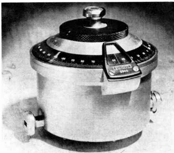
Figure 5. Standing wave indicator for covering the complete 8 mm band. Outer scale sets frequency, inner scale measures phase. Performance matches that of best slotted sections but simplicity makes unit much cheaper.
