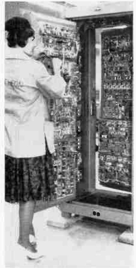
Raytheon Canada Limited employee Lola Wrobel shown above makes final cable adjustment to Bright Display System which converts radar signals into television form. Units are being produced at the company's new headquarters' plant at Waterloo, Ontario. The Bright Display System makes Canada's trans-continental long range surveillance network even more efficient.
