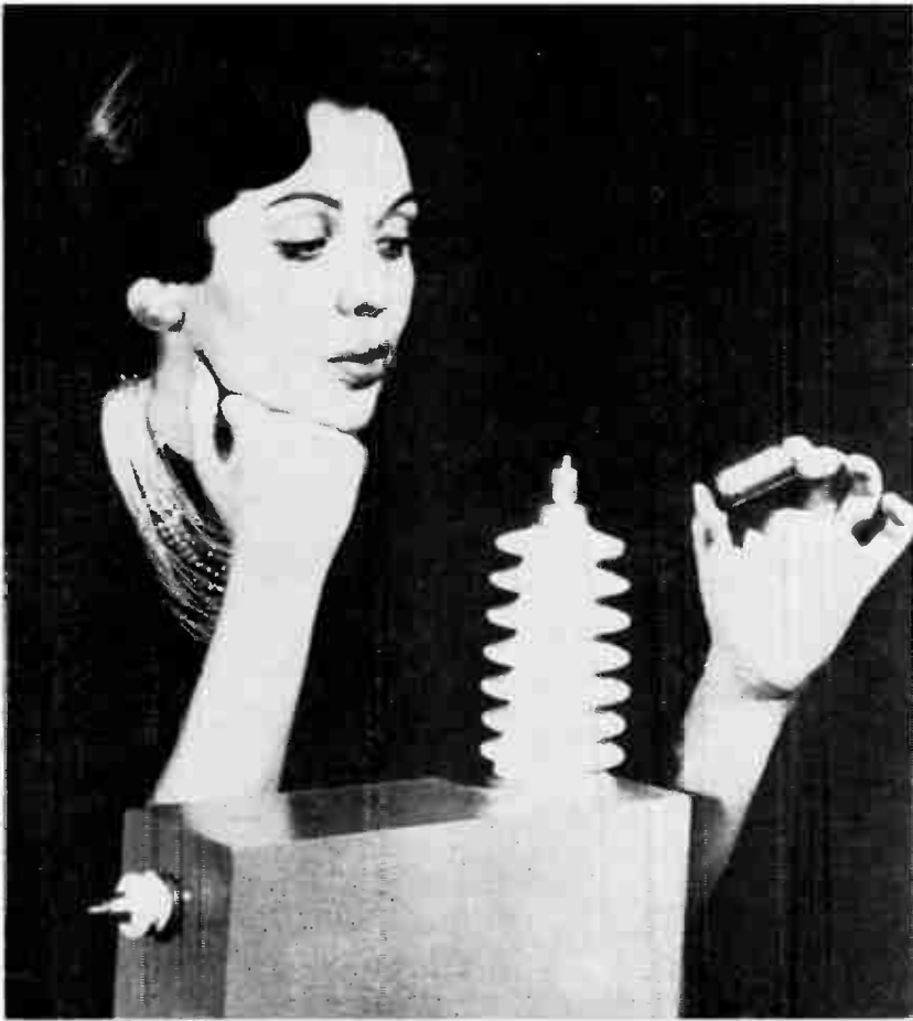
This is probably the largest precision resistor voltage divider built to date. Made by Resistance Products Co. of Harrisburg, Pa., for a Texas firm (everything's bigger in Texas), this network was built on special order as a precision 30 megohm 100 to 1 divider to operate at 30,000 volts with .05 accuracy. (The small resistor being held by the attractive Miss is solely for the purpose of comparison.)
